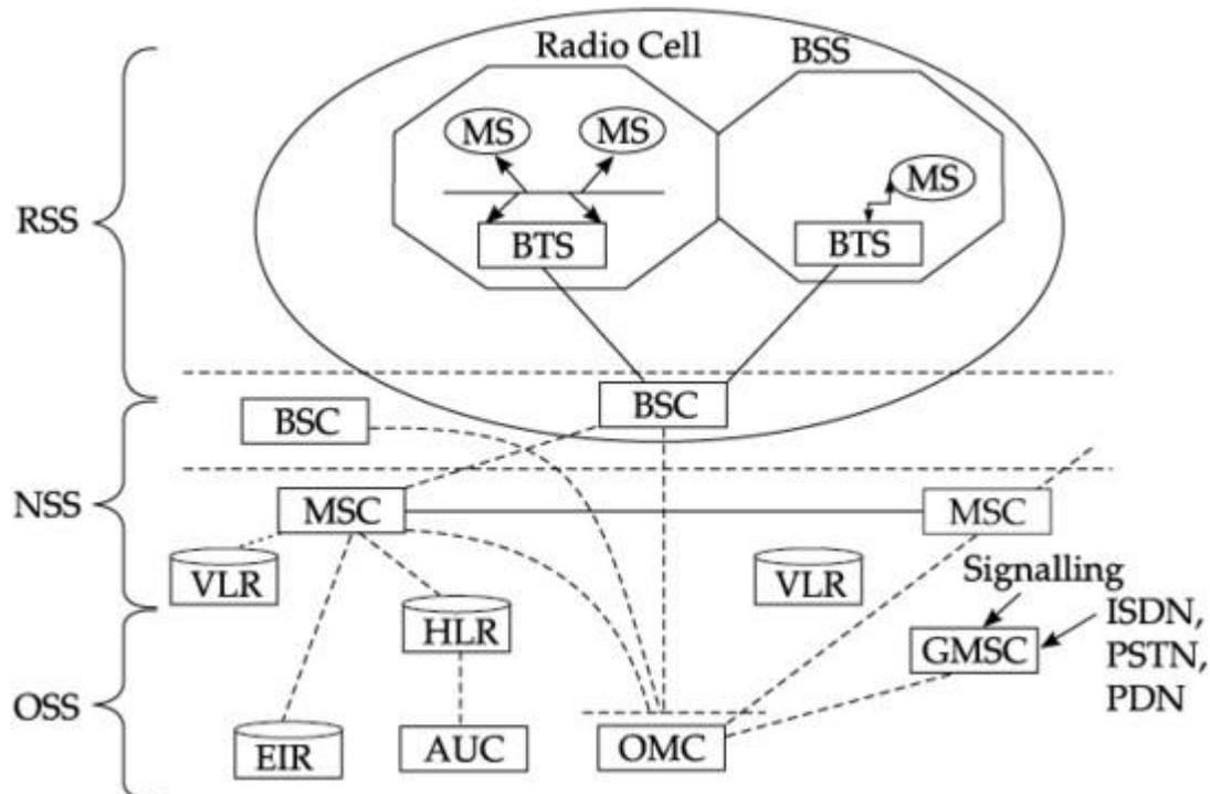
**Figure 2.1.2 Functional Architecture of a GSM System**
