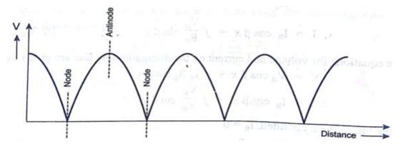
Nodes are the points of zero voltage or current and anti-nodes are the points of maximum voltage or current in the standing wave systems.
