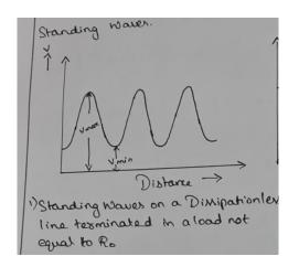
The plot of current variation along the line is the same as that of voltage variation except for a  $\frac{\lambda}{4}$  shift in the position of maxima and minima.
