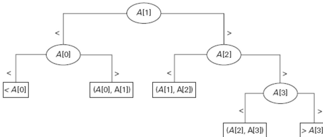
$$C_{\text{worst}}(n) \geq \lfloor \log_2(n + 1) \rfloor$$
