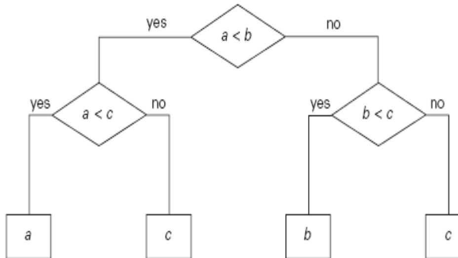
Each internal node of a binary decision tree represents a key comparison indicated in the node, e.g.,  $k < k$ . The node's left subtree contains the information about subsequent comparisons made if  $k < k$ , and its right subtree does the same for the case of  $k > k$ . Each leaf represents a possible outcome of the algorithm's run on some input of size  $n$ .
