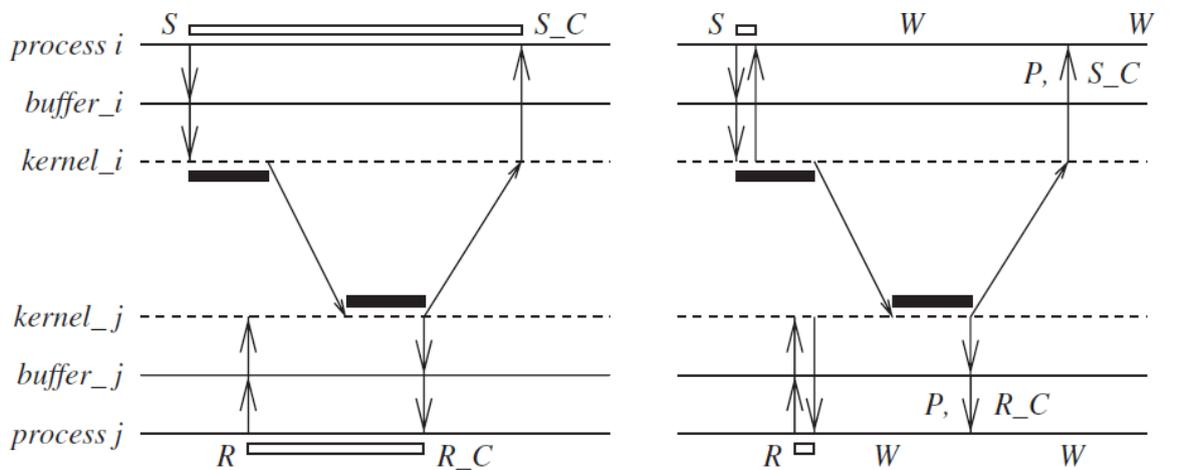
(a) Blocking sync. Send, blocking Receive      (b) Nonblocking sync. Send, nonblocking Receive
