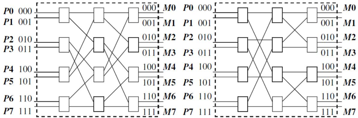
(a) 3-stage Omega network ( $n = 8, M = 4$ )      (b) 3-stage Butterfly network ( $n = 8, M = 4$ )
