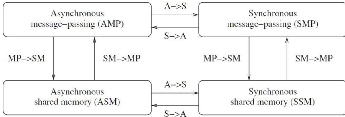
*Figure 1.11 Emulations among the principal system classes in a failure-free system*
