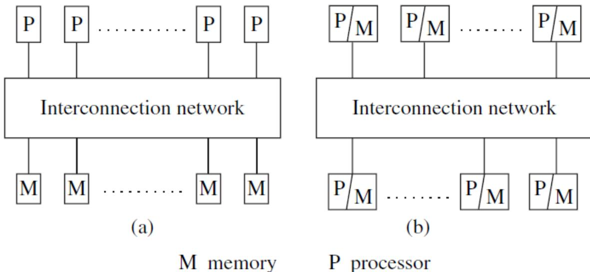
**Figure 1.3** Two standard architectures for parallel systems. (a) Uniform memory access (UMA) multiprocessor system. (b) Non-uniform memory access (NUMA) multiprocessor. In both architectures, the processors may locally cache data from memory.
