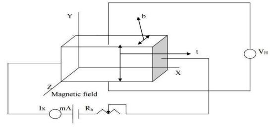
This sample is placed in between two poles of an electro magnet such that magnetic field is applied along Z –axis.
